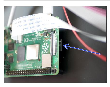
Insert the Micro SD card into the Raspberry Pi and power up your printer.
