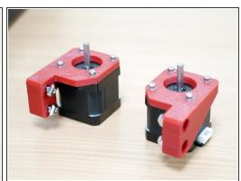
Take the two motors from the old Top Panel Assembly. The motor number should have a 205 in it.
