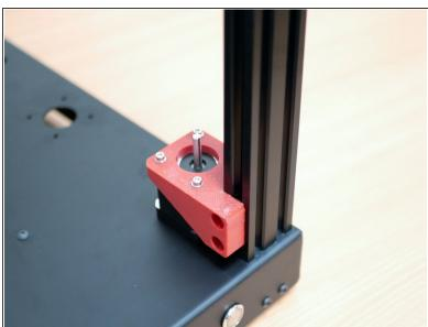
(i) Secure those motor assemblies to the inside front of the frame as shown.
