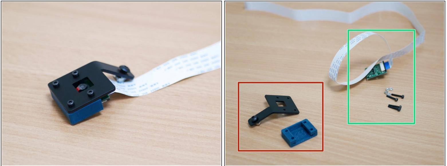
**i** Detach the old Pi Cam assembly from the printer and disassemble it.
