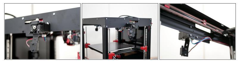
(i) Remount the extruder assemblies to the sides of the frame.
