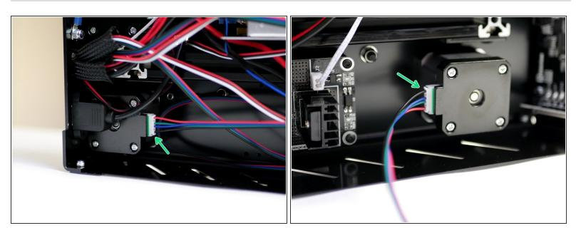
Connect motor cables to both Z-motors.
