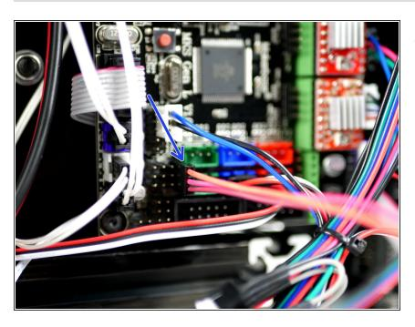
Connect the servo cable to the electronics board like shown.
