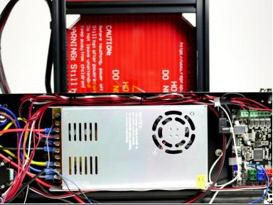
(i) Cable tie the print fan cables to the Hotend cables and tuck away.
