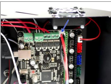
Connect both cables form the print fans to the print fan adapter.
