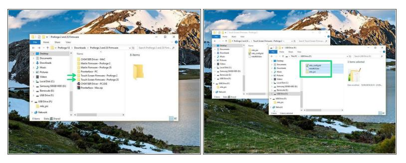
Copy the contents of the Touch Screen Firmware folder (depending on whether you're building a Proforge 2 or 2S) to the included SD card.
