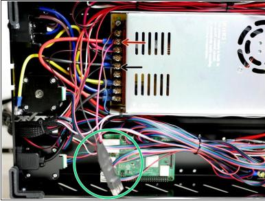
Connect the USB convertor to the power supply.
