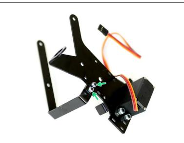
Install the second print fan mount with two M3 x 8mm bolts and M3 Nyloc nuts.
