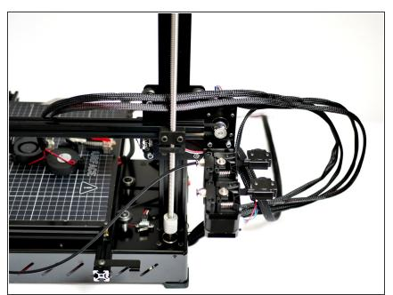
(i) Remove all of the cable ties from the main branch of cables going down to the base.
