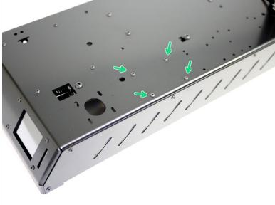
• Fix four M3 x 15mm standoffs to the base with four M3 x 6mm bolts.
