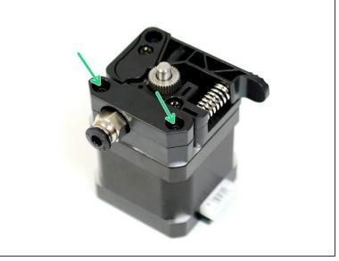
• Fix the Coupling Bracket onto the motor with two M3 x 16mm bolts.
