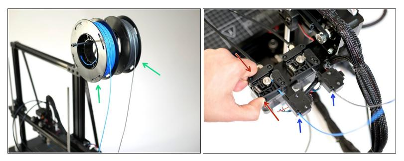
• Place a spool of filament onto both of the spool holders.
