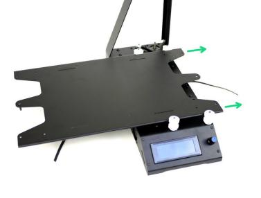
Slide the platform onto the guides from the left side, like shown.
