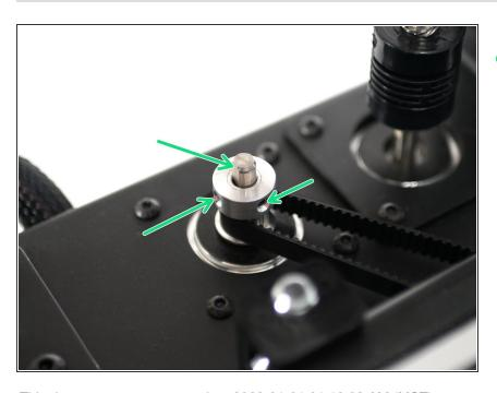
Secure the pulley onto the flat side of the motors shaft.
