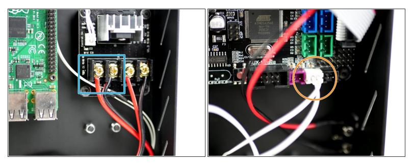
• Connect the heated bed power cables to the MOSFET terminals like shown.
