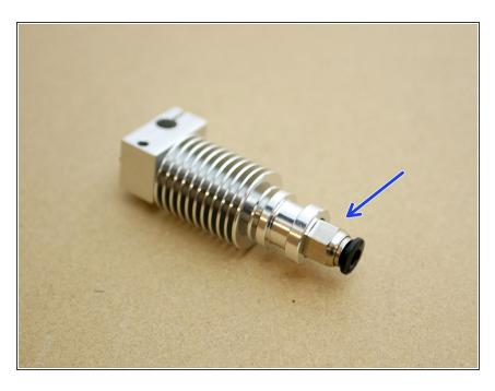
Fix the pneumatic coupling onto the Heatsink.
