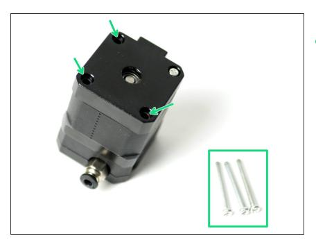
Remove from the back of the extruder motor three of the bolts.
