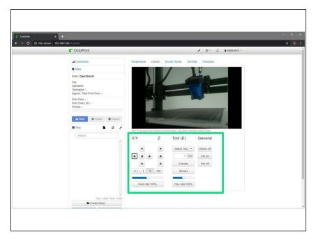
Check that you can move the axes of the printer with the Octoprint control panel.
