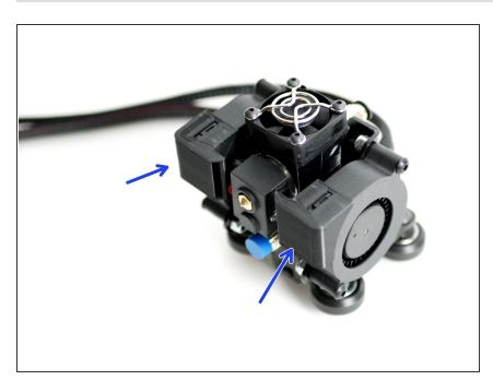
• Snap both of the 3D Printed Fan Shrouds onto the Blower Fans.
