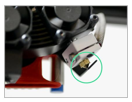
Adjust the ooze shields by bending the metal sleds until they are able to make contact with the tips of both nozzles.
