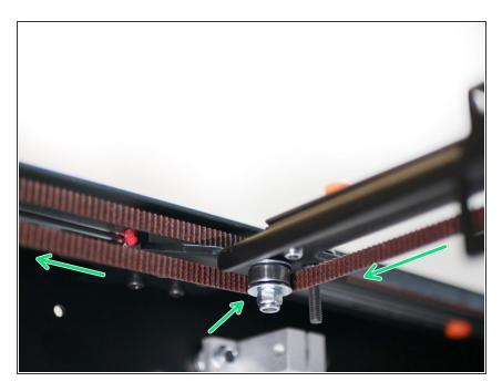
Take the left side of the belt and wrap it around the lower left idler on the gantry as shown.
