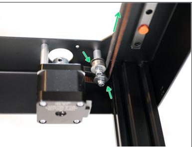
As before, wrap the belt around the motor pulley first and then around the two rear right idlers like shown.
