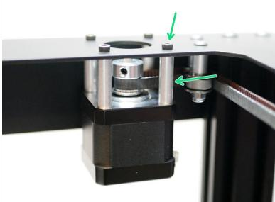
Refit the motor bolts and spacers.
