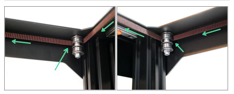
Whilst keeping some tension on the belt to prevent it from falling off the idlers, pull it forward and wrap it around the front idlers like shown.
