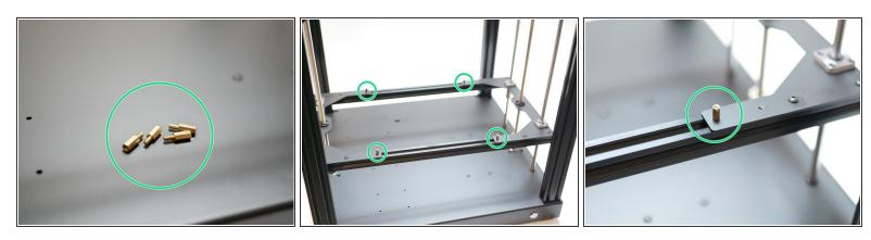
Take the four M3 brass stand-offs and secure them onto the platform assembly as shown.
