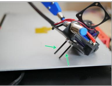
Replace the M3 x 25mm bolts on the metal tool carriage with the two M3 x 35mm bolts.
