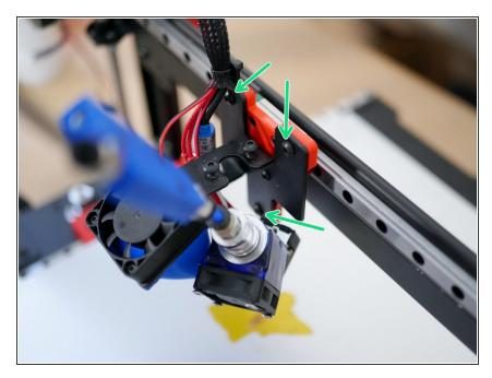
Mount the metal tool carriage onto the 3D printed one with three M4 x 6mm bolts.
