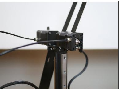
(i) Finally, re-attach the belt and the extruder.
