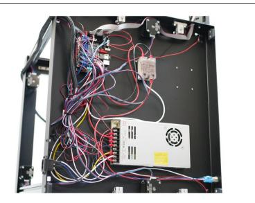
Finally, use cable tie mounts to clean up the cables.
