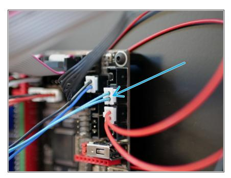
Connect the thermistor to the control board.
