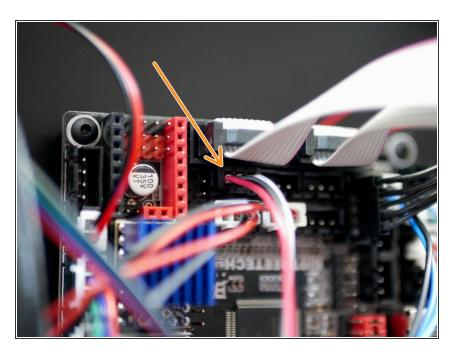
Connect the filament sensor to the control board as shown.
