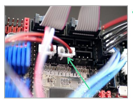
Connect the Y-Endstop to the control board.
