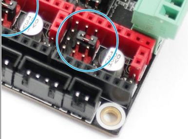
• Make sure the jumpers under the steppers are positioned as shown.
