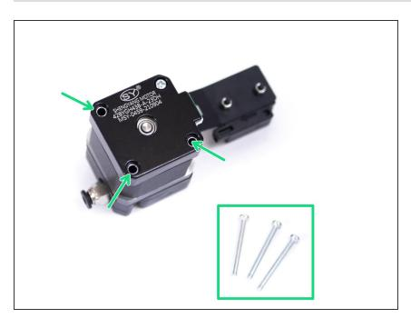
From the rear of the NEMA 17 motor remove three of the four bolts as shown. Stage 03: Extruders Guide ID: 99 - Draft: 2022-05-20
